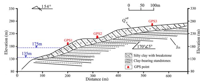
**Figure 3.** 1–1' geological section of Wangmiao landslide.
