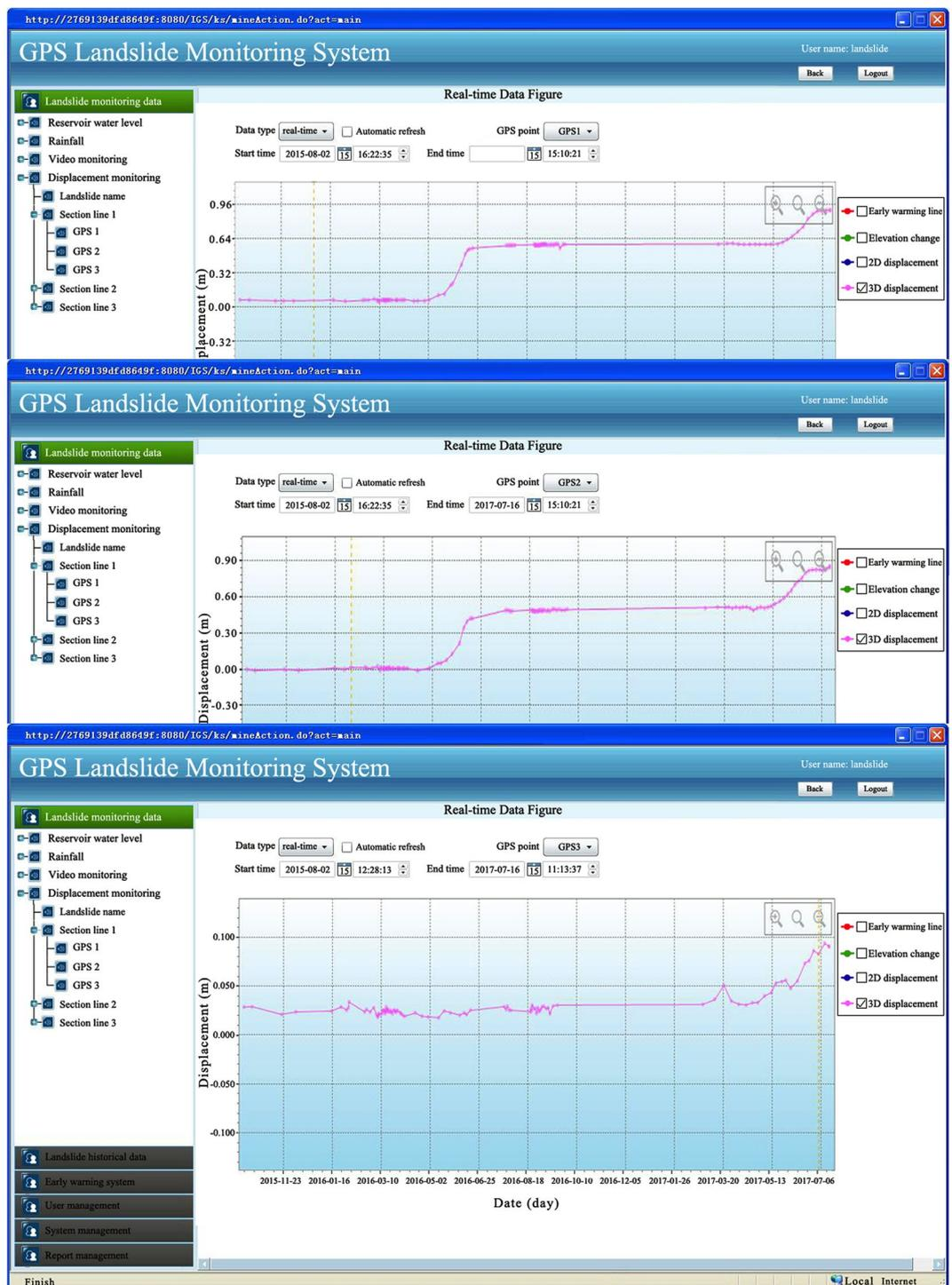
**Figure 6.** GPS 1, GPS 2 and GPS 3 monitoring landslide displacements.
