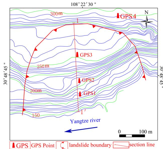
**Figure 2.** Geographical location map of the Wangmiao landslide (AUTOCAD 2014, <https://www.autodesk.com.cn/>, drawn by Faming Huang).
